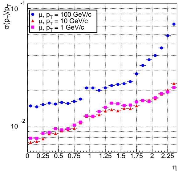
Figure 2: Transverse momentum resolution for single muon events with  $p_T = 1, 10, 100 \text{ GeV}/c$  as a function of  $|\eta|$ .
