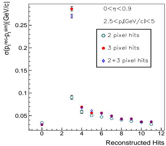
Figure 4:  $P_T$  resolution as a function a number of reconstructed hits in the barrel compared to the full tracker performance (the leftmost point at “0”).
