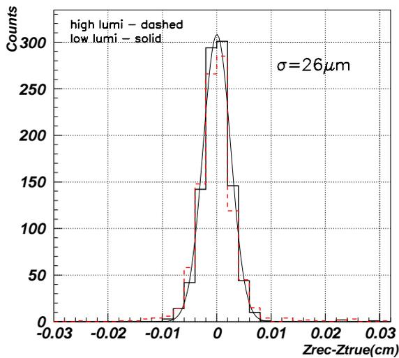
Figure 3: Difference in the  $z$  position between the reconstructed and the simulated vertex at low and high luminosity. The standard deviation of the Gaussian fit is quoted as the resolution on the primary vertex position.
