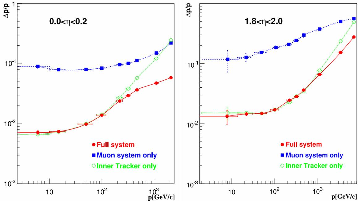
Figure 2: Resolution of  $1/p$  vs.  $p$  for standalone, global and tracker-only muon reconstruction in the (left) barrel and (right) endcap regions.
