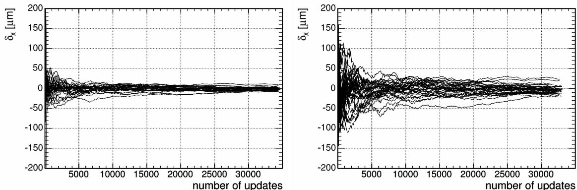
Figure 3: Kalman filter algorithm: evolution of the differences between the estimated and the true local  $x$ -shifts in (left) layer 1 and (right) layer 2 of TIB.
