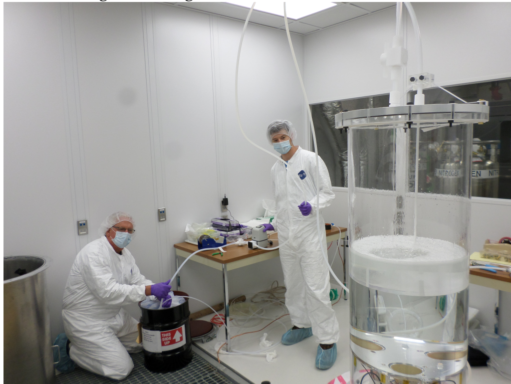
GdLS filling in underground cleanroom
