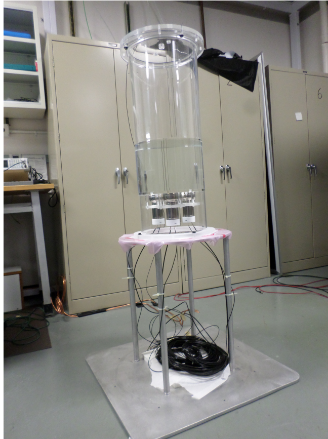
PMTs mounted and cabled (detector stand designed by Susanne)
