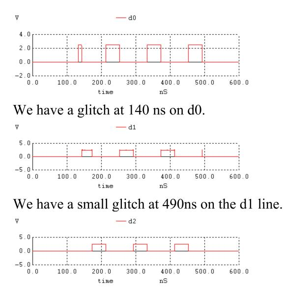
The Pixel readout is shown below decoded;
