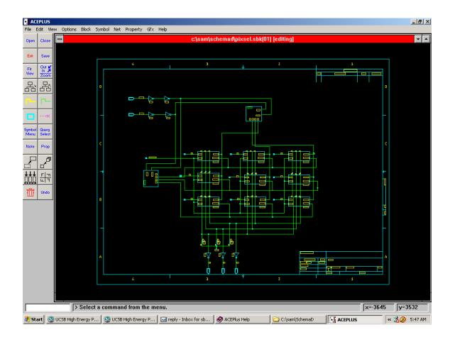
A Feedback FB input was added to 3bit columb and row shift registers and r3 from row register is used as the clock for the columb register, r3 from the row register is also fed back to the
