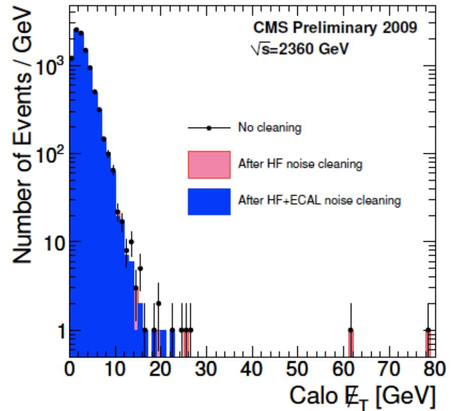
HF “noise” may be due to particles directly hitting the window of HF PMT;
