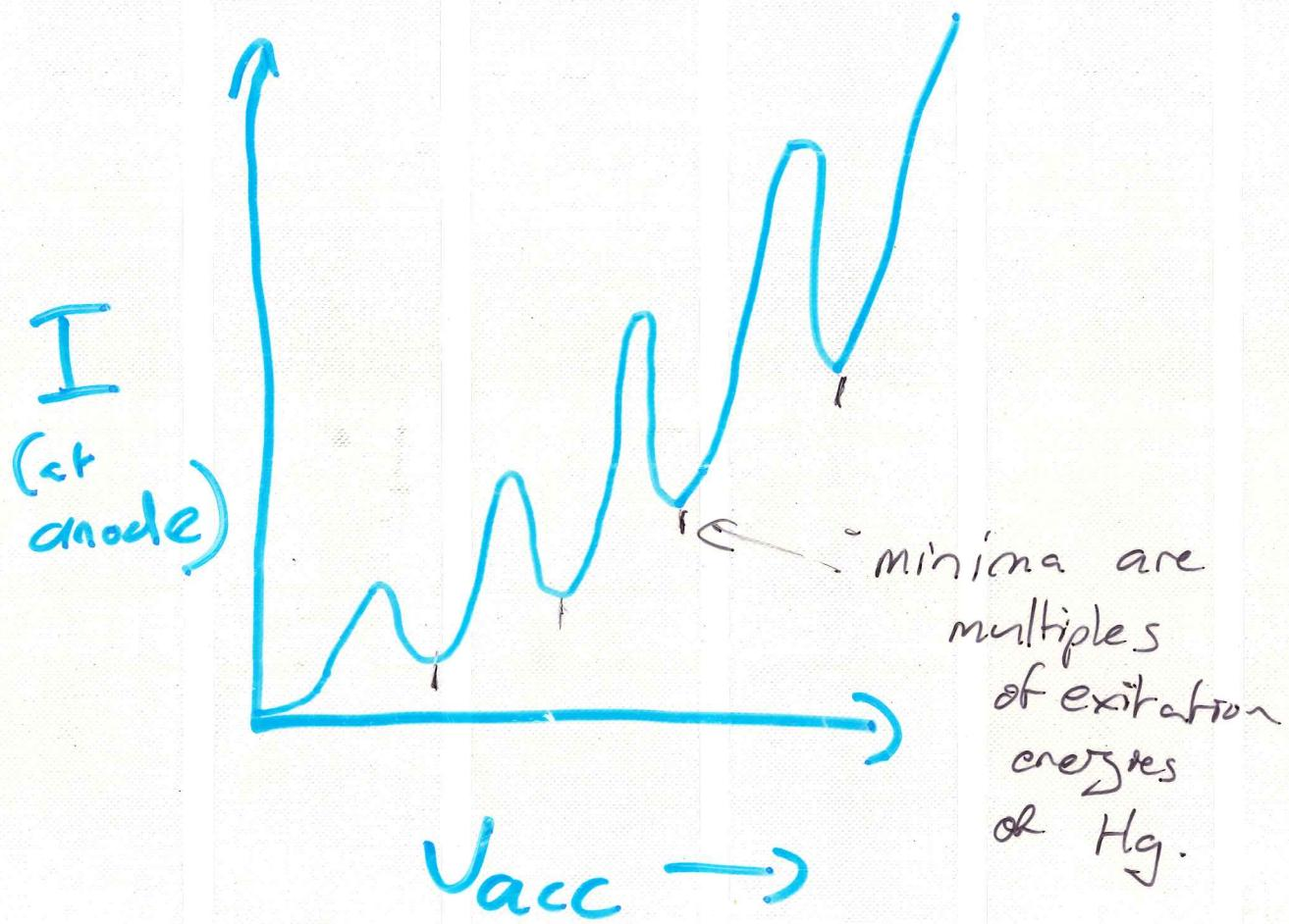
When the electrons have energies at (or above) the excitation energies of Hg, they can lose energy in multiples of the excitation energy.
