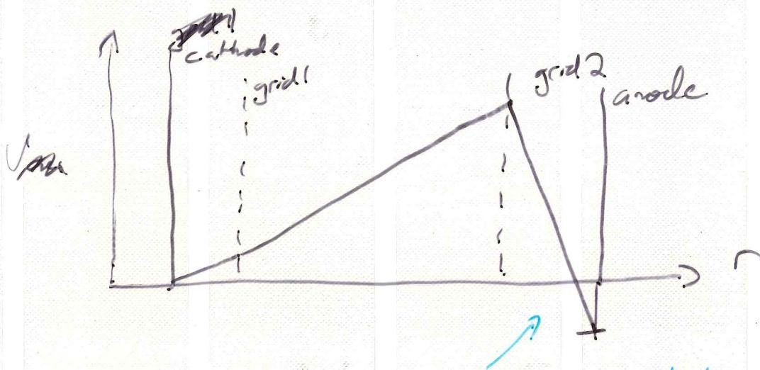
note the total voltage drops between the cathode and the anode. No electrons can get through.
