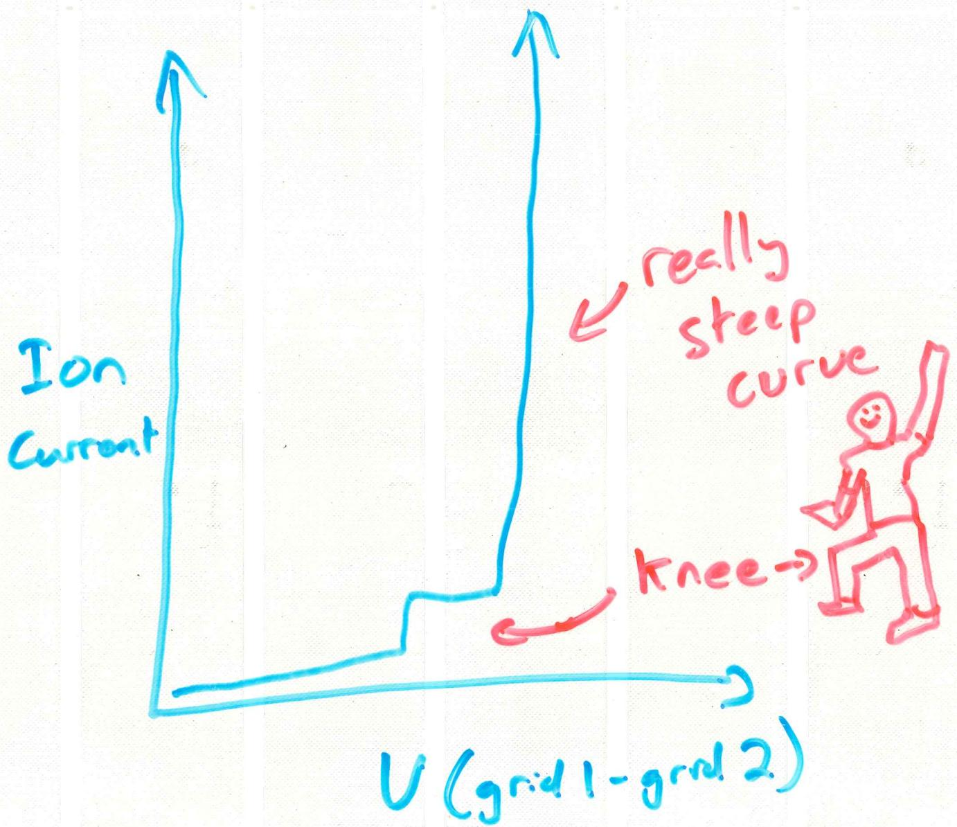
The knee is due to the photo-electric effect (excited mercury atoms give off UV photons when they fall back to the ground state. Those photons hit the anode, and the loss of negative electrons creates the same sort of currents as a gain of positive ions.)
