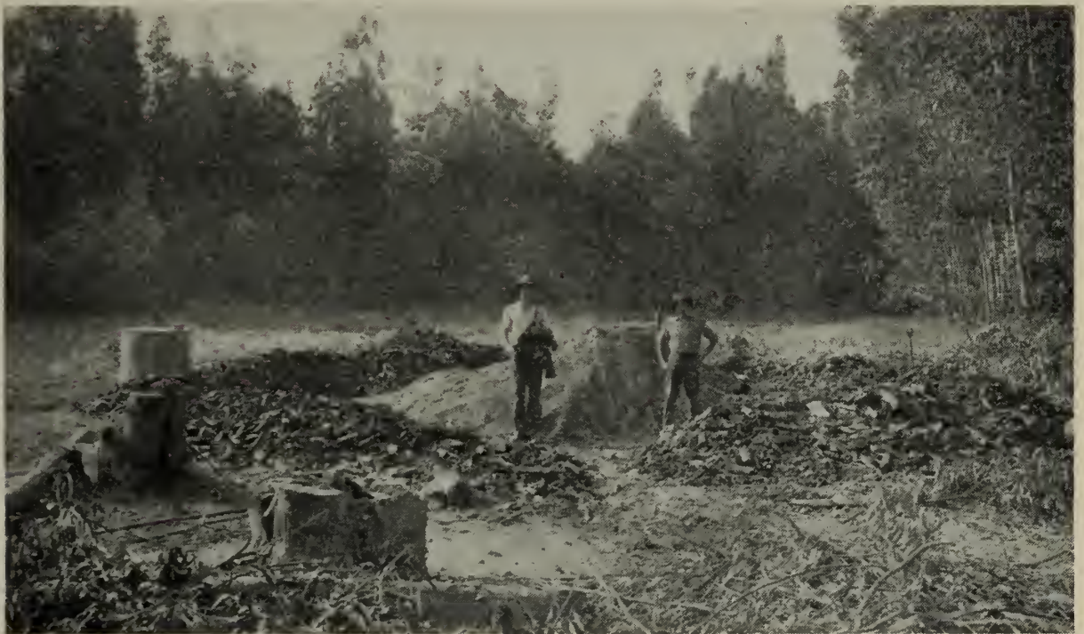
Fig. 24.—A pile of charcoal from 25 cords of Eucalyptus wood burned in an earth kiln for 21 days. When handled in this way it produces about 1000 pounds of charcoal a cord.
