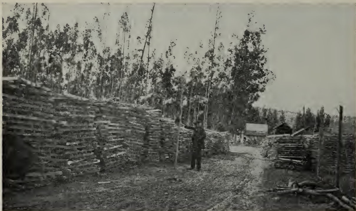
Fig. 23.—These pieces of Blue Gum are 1\frac{7}{8} inches square by 6 feet long, cut from a grove at Stony Point, Sonoma County. Blue Gum is suitable for the manufacture of insulator pins and other small turned articles. After being seasoned for six to eight weeks in open piles these blanks are turned into insulator pins, the product averaging about 2500 pins a cord. A stumpage price of $4.50 a cord has been paid for 25-year-old groves used for this purpose.
