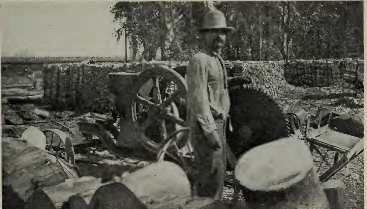
Fig. 22.—A gasoline engine saw outfit cutting 12-inch cordwood from a Blue Gum grove 15 years old, near Sanger, Fresno County. The crew of three men can cut 7\frac{1}{2} cords a day at a cost of about $8.00 a cord for felling, sawing and stacking. The wood sells for $14.00 to $16.00 a cord at the grove.
