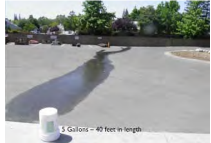
Five gallon spill on sloped surface
