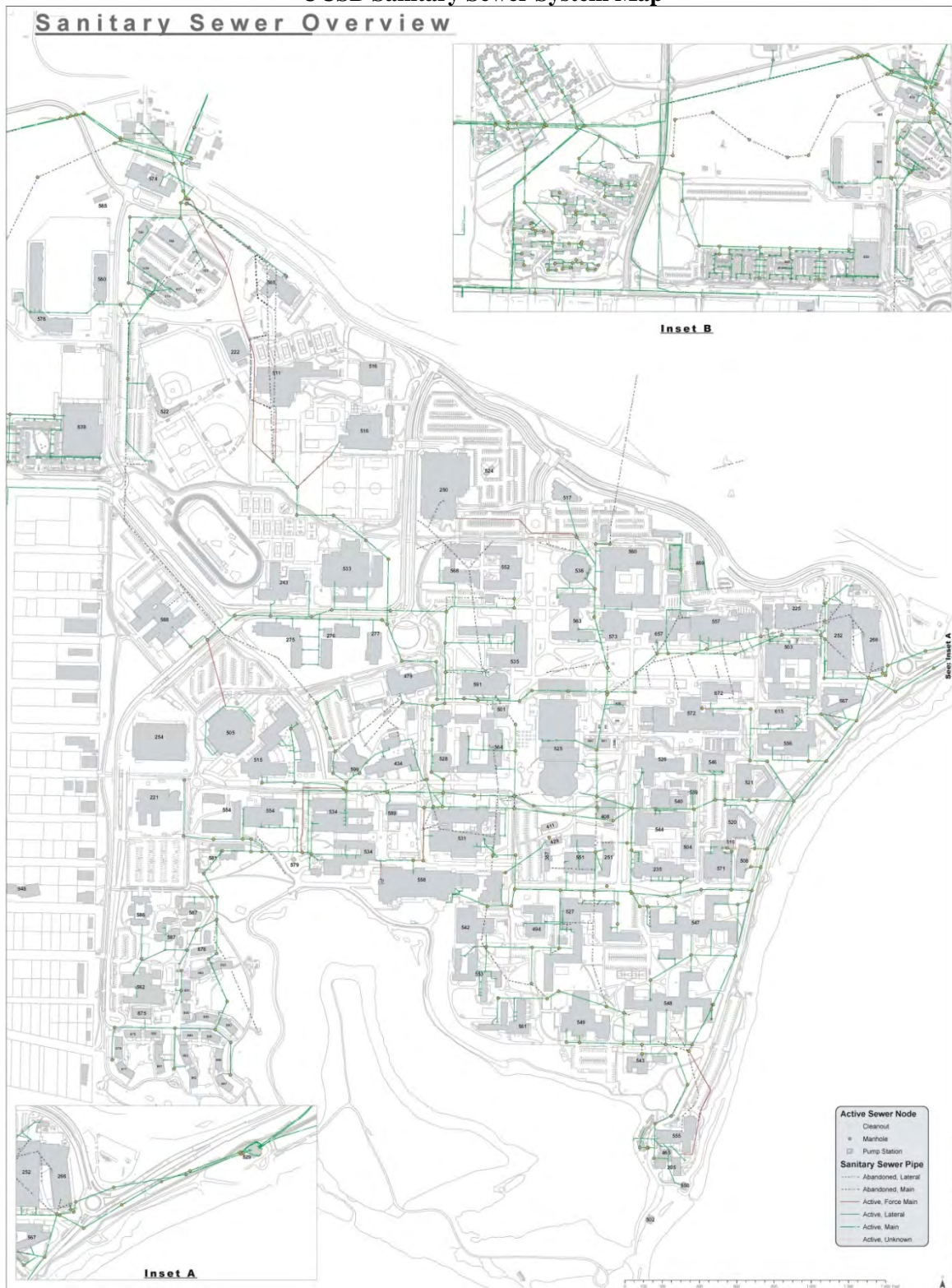
Figure 2-2 UCSB Sanitary Sewer System Map
