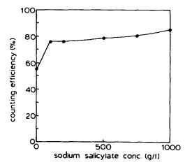
FIG. 3. Counting efficiency as a function of the concentration of the wavelength shifter sodium salicylate. Counting conditions as described in the caption to Fig. 2.
