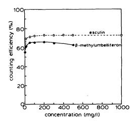
FIG. 2. Counting efficiency as a function of the concentration of wavelength shifters esculin and  $\beta$ -methyl umbelliferon. Polyethylene vials, content 10 ml; Na<sub>2</sub>H<sup>32</sup>PO<sub>4</sub> in distilled water at pH 7.0; amplifier gain 30%.
