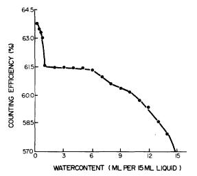
FIG. 8. Detection efficiency of <sup>32</sup>P-Čerenkov radiation in ethanol and the effect of increasing amounts of water.
