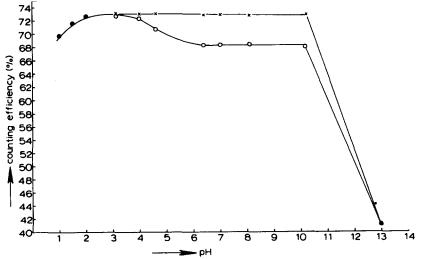
FIG. 6. The effect of pH on the function of the wavelength shifter esculin. (×) measured immediately after preparation of the samples; (O) measured upon two weeks storage of the samples. 400 mg esculin/l; counting conditions as described in the caption to Fig. 2.
