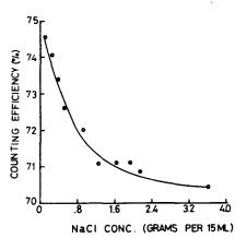
FIG. 4. The effect of salt on the function of the wavelength shifter sodium salicylate. Sodium salicylate concentration 200 g/l. Other counting conditions as described in the caption to Fig. 2.
