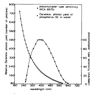
FIG. 1. Comparison of Čerenkov photon yield and spectral response of a typical photomultiplier tube used in a commercial liquid scintillation counter.
