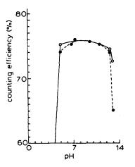
FIG. 7. The effect of pH on the function of the wavelength shifter sodium salicylate. (O) measured immediately after preparation of the samples; (•) measured upon two weeks storage of the samples. 200 g/l sodium salicylate; other counting conditions as described in the caption to Fig. 2.
