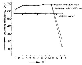
FIG. 5. The effect of pH on the function of β-methyl umbelliferon as wavelength shifter. (×) measured immediately after preparation of the samples; (O) measured upon two weeks storage of the samples.
