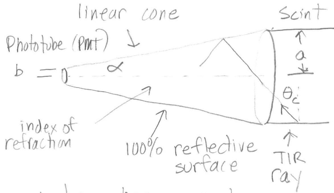
Can  $\alpha$  be chosen such that  $100\%$  of Totally Internally Reflecting (TIR) rays hit the phototube (PMT) ?
