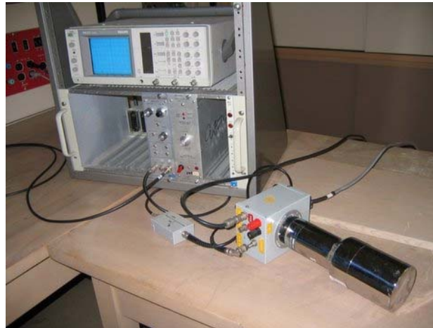
typical NaI(Tl) detector in Queen's undergraduate lab
