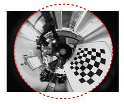
**Figure 2:** An example calibration image. The predicted image of the outer mirror rim, presented by the dashed circle, coincides with the actual outer rim that is partially visible in the image.
