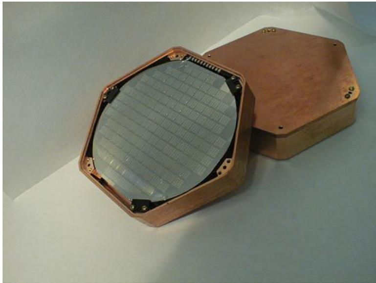
Figure 2.1: A photo of a ZIP detector. Shown is the phonon channel side. Each ZIP is 1 cm thick, and 7.62 cm in diameter.
