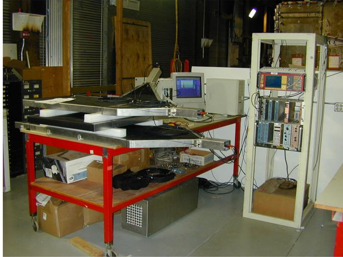
Figure 6.1: Digital photo of the muon telescope, also shown is the DAQ electronics with a charge spectrum displayed on the computer.
