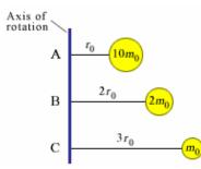
The figure shows three objects rotating about a vertical axis. The mass of each object is given in terms of  $m_0$ , and its perpendicular distance from the axis is specified in terms of  $r_0$ . Rank the three objects according to their moments of inertia, **largest to smallest**.
