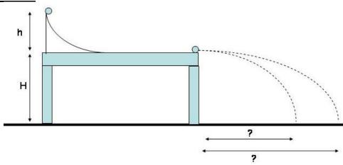
A marble of mass 2m slides down a frictionless incline which is placed on a table as shown in the figure. This marble then strikes a second marble of mass m. The two marbles then hit the floor below.
