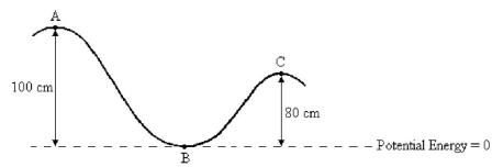
A 2.0-g bead slides along a wire, as shown in the Figure. At point A, the bead is at rest. Neglect friction and use  $g = 10 \text{ m/s}^2$ . What is the speed of the bead at point B?
