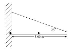
A store's sign, with a mass of 20.0 kg and 3.00 m long, has its center of gravity at the center of the sign. It is supported by a loose bolt attached to the wall at one end and by a wire at the other end, as shown in the Figure. The wire makes an angle of 25.0° with the horizontal. What is the tension in the wire?
