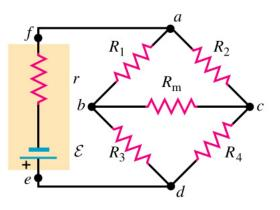
For example:  $V_{ab} + V_{bc} + V_{ca} = 0$   $(V_a - V_b) + (V_b - V_c) + (V_c - V_a) = 0$ But this holds for any loop, e.g. a-b-d-c-a or b-a-f-e-d-b, .....
