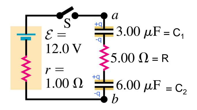
Equivalent capacitance:  $1/C_{eq} = 1/C_1 + 1/C_2 \rightarrow C_{eq} = 2 \ \mu F$ Series resistance  $R_{eq} = r+R = 6 \ \Omega$
