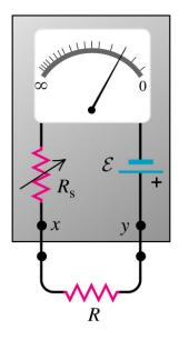
Galvanometer as a resistance meter (aka Ohmmeter)
