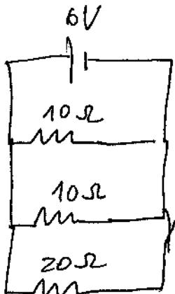
$$(c) \text{Req} = \frac{1}{\frac{1}{R_1} + \frac{1}{R_2} + \frac{1}{R_3}} = \left( \frac{1}{10} + \frac{1}{10} + \frac{1}{20} \right)^{-1}$$
