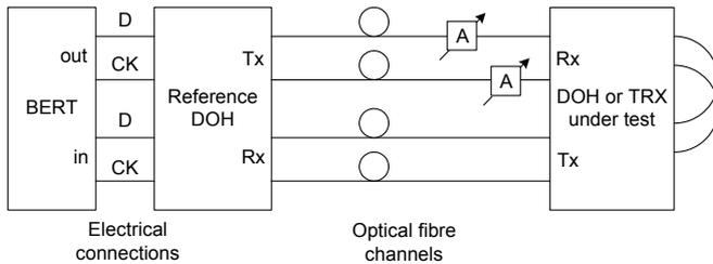
Figure 5: Receiver test-setup.
