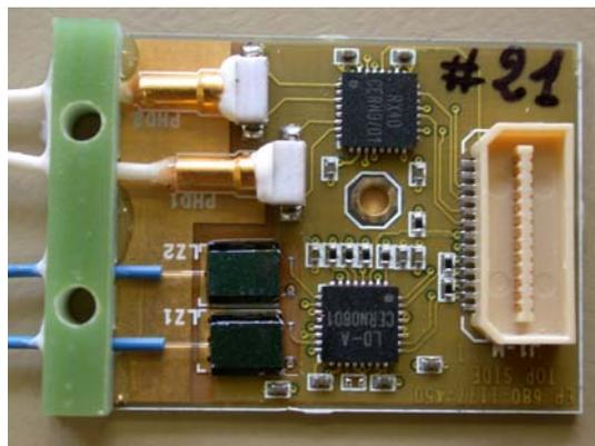
Figure 2: Photograph of prototype DOH showing the back-side containing the active parts. Left: two photodiodes above 2 laser diodes. Middle: packaged RX40 and LLD ASICs connected to the photodiodes and lasers respectively. Right: male 26-way NAIS connector, the electrical interface to the ring of CCU's in the Tracker. Several capacitors are mounted on the front-side.
