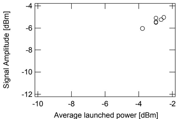
Figure 3: Transmitter optical output characteristics on the 3 DOHs tested. The measurements were made with the existing default I2C settings of the LLD ASIC at power-up of the DOH. These are 22mA dc bias and 12.5mS gain.
