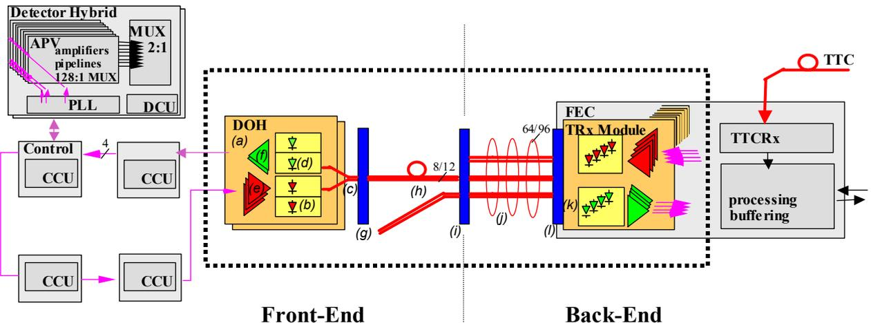
Figure 1: CMS Tracker control ring[1]. The front-end is exposed to radiation, a 4T magnetic field, and will operate at  $-10^{\circ}\text{C}$ . The labels (a) through (l) correspond to references in the text.
