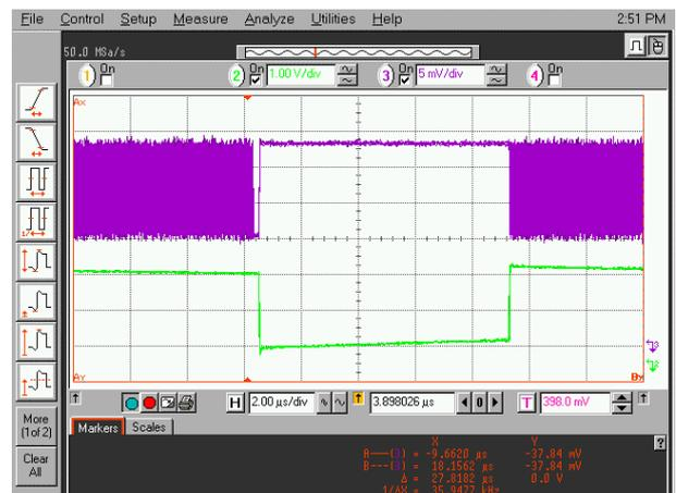
Figure 8: Reset action of RX40. The upper Trace is the input data signal where a train of 10 zero-levels generates a reset flag (lower trace) from the RX40. The data output is disabled during the period that the reset flag is set 'low'.
