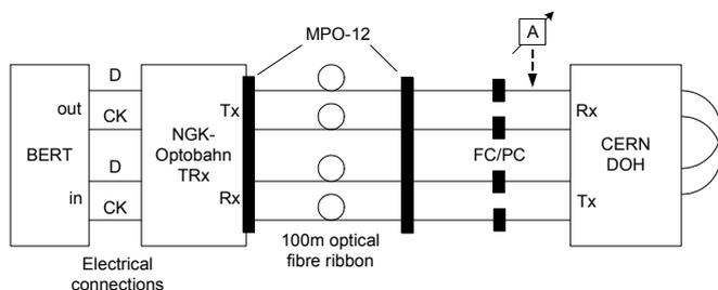
Figure 9: Full link test set-up.
