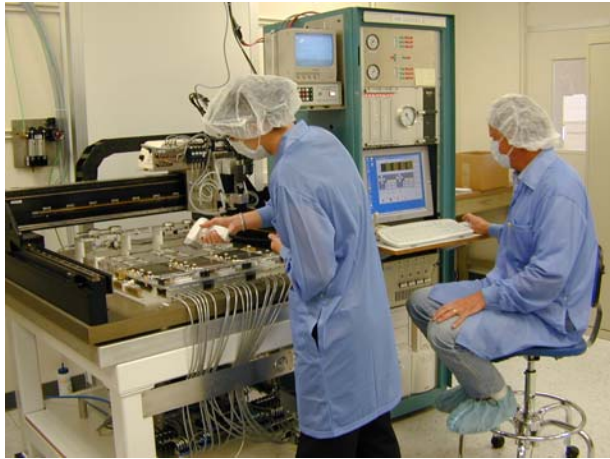
Gantry makes modules (30/day)
