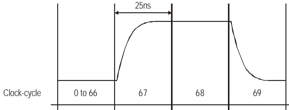
**Figure 2-2 Ideal waveform of the Tick-Mark**
