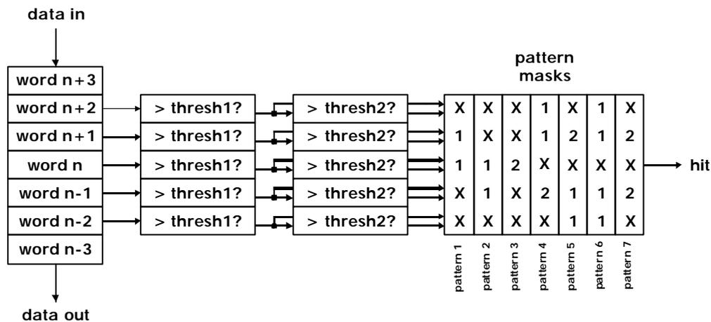
**Figure 3-4 Practical Implementation of the Cluster Finding Algorithm**
