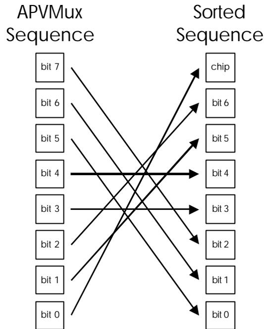
**Figure 3-3 APV output bit-swapping sequence**
