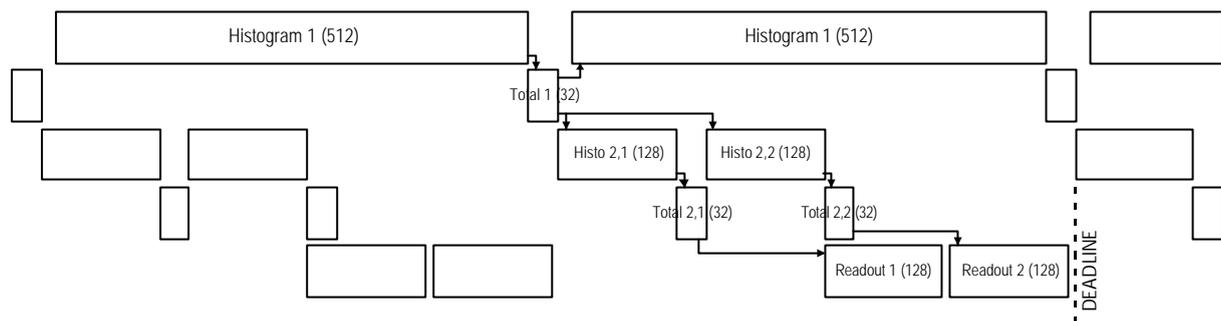
**Figure 3-2 Timing Diagram for Median Calculation**
