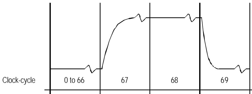
**Figure 2-3 Non-ideal waveform of the tick-mark**
