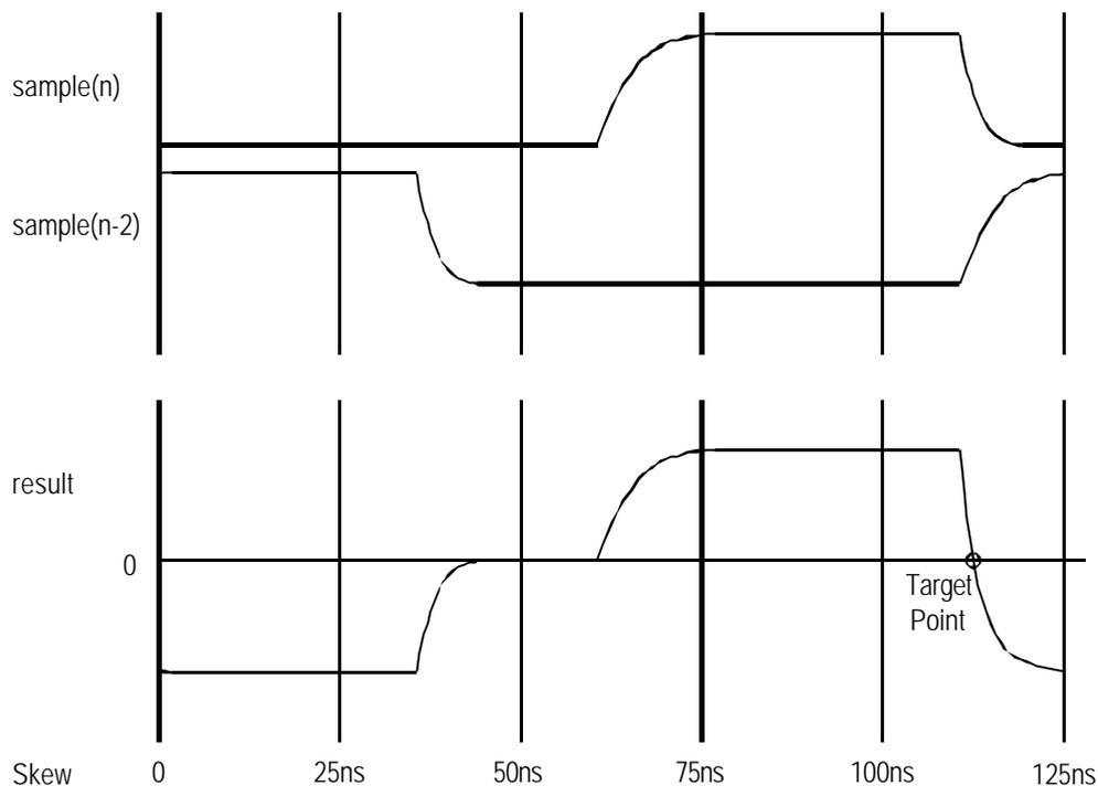
**Figure 2-4 Result of averaging the difference between alternate ADC samples**
