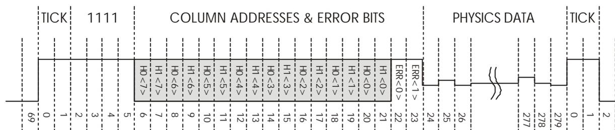
**Figure 2-7 APV Frame (40MHz interleaved)**
