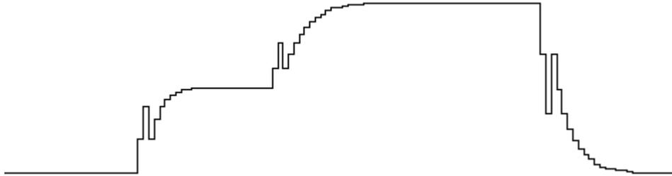
**Figure 2-5 Result Waveform produced using non-ideal Clock Vernier**
