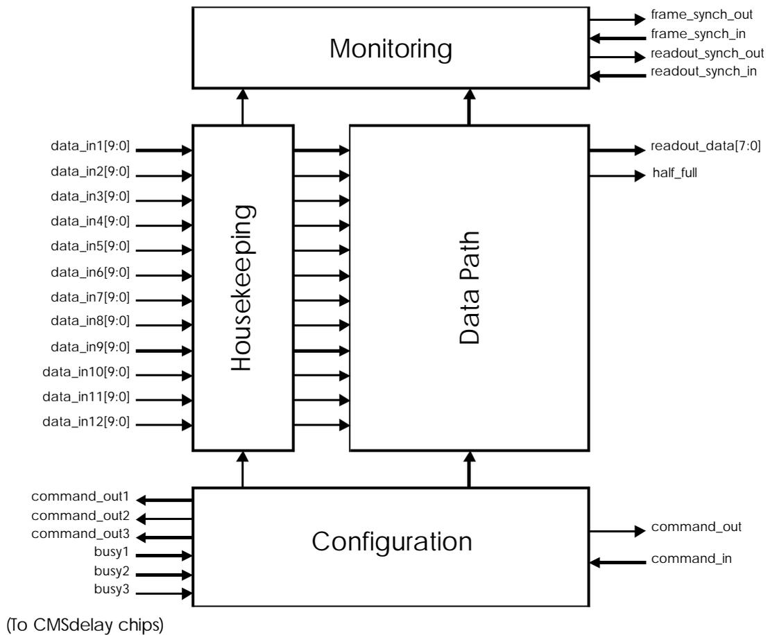
**Figure 1-1 Block Diagram of the Front-End FPGA**
