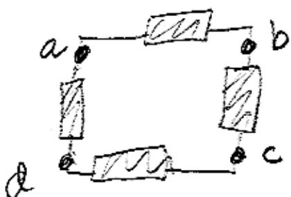
$$V_{ab} + V_{bc} + V_{cd} + V_{da} = 0$$
