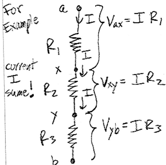
$$\begin{aligned} V_{ab} &= V_{ax} + V_{xy} + V_{yb} \\ &= IR_1 + IR_2 + IR_3 \end{aligned}$$
