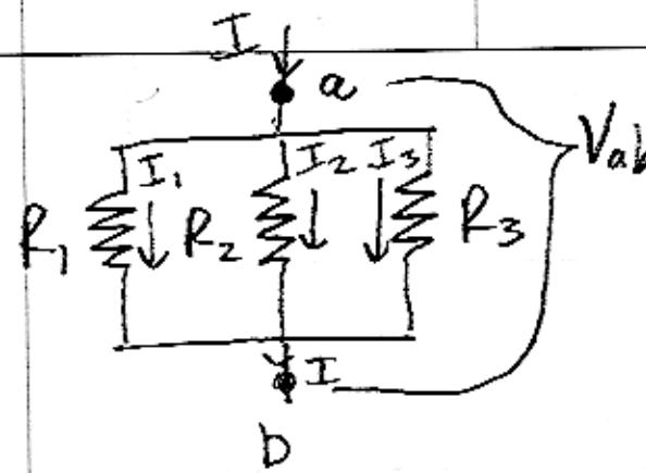
$$V_{ab} = I_1 R_1 = I_2 R_2 = I_3 R_3$$
