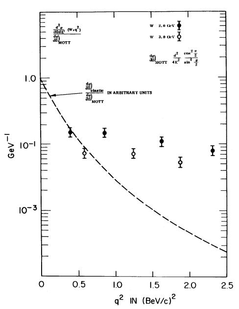
Fig. 11. Inelastic data for W=2 and 3 GeV as a function of  $q^2$ . This was one of the earliest examples of the relatively large cross sections and weak  $q^2$  dependence that were later found to characterize the deep inelastic scattering and which suggested point-like nucleon constituents. The  $q^2$  dependence of elastic scattering is shown also; these cross sections have been divided by  $\sigma_M$
