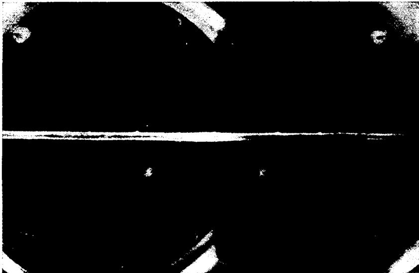
Fig. 8. A positive-negative electron pair (energies of negative and positive 4.6 and 140 million electron-volts respectively) generated in the gas (argon) of the chamber by a photon associated with the cosmic rays. (Magnetic field 7,900 gauss.)
