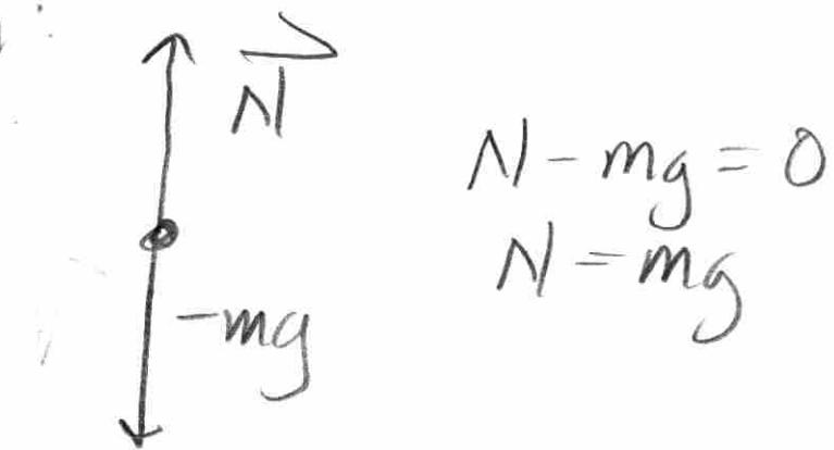
Neither  $\vec{N}$  nor  $-mg$  do any work, because the displacement  $\vec{s}$  is  $\perp$  to these forces.
