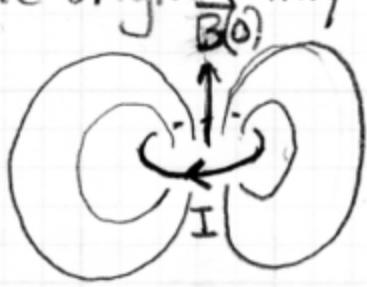
$$\vec{B}_{\text{far}} = \frac{1}{r^3} \left[ \frac{3(\vec{\mu} \cdot \vec{r})\vec{r}}{r^2} - \vec{\mu} \right] \times \frac{\mu_0}{4\pi}$$
