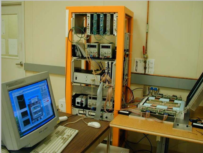
Hybrid thermal cycler in the Lab D clean room
