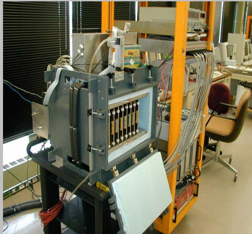
LT system with brass insertion plates (one of two sets) at Fermilab
