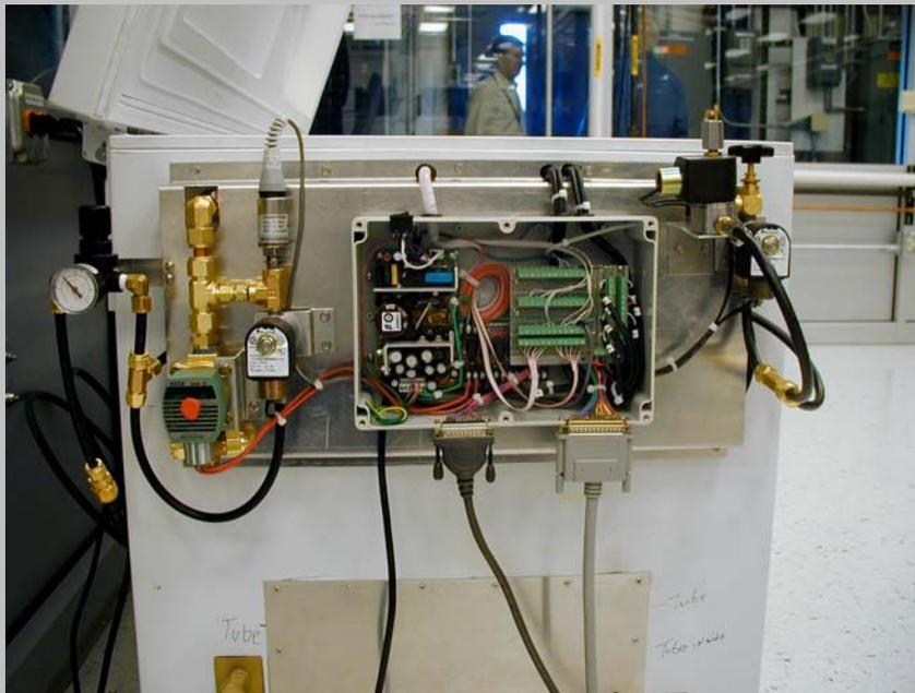
**Input and output manifolds allow constant pressure differential across variable number of rods**
