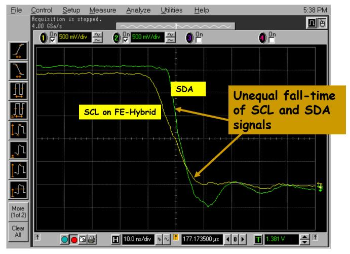
Picture shows sequence of SCL/SDA signals with SDA pulled-down in AOH and measured on FEH I2C bus on TOB A.M.
