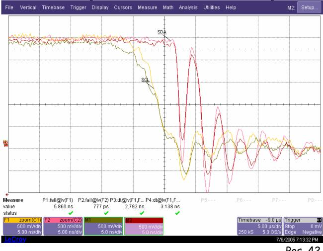
Pos. 42 LDD response measured on the AOH at -23°C and at RT W. Karpinski-Aachen 14
