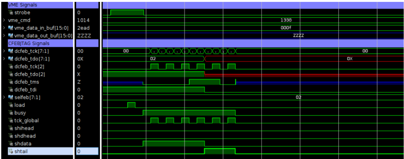
Figure 9: Simulated ODMB response to VME command W 1338 000F. In this example, xDCFEB 2 is selected. The tdo signals are unimportant and may differ for real xDCFEBs.
