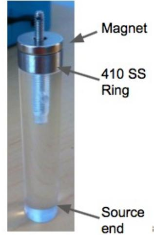
**Figure 7.2.4:** Prototype dummy source capsule showing 410SS ring with magnetic recovery system attached.
