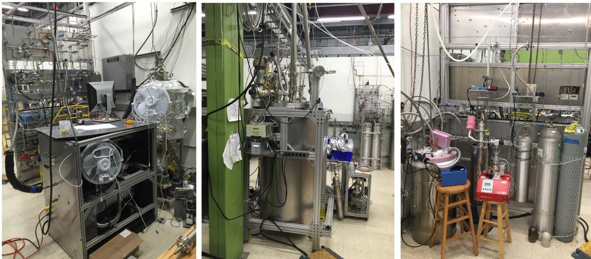
**Figure 6.3.1:** The three panels show the Kr removal development platform. Left: the gas control manifold, pumps, and charcoal column. Center: LN thermosyphon cooled condenser for xenon recovery. Right: krypton traps and xenon feed and storage located on the back side of the manifold.
