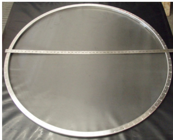
Figure 6.2.1.7. A 1.16-m-diameter stretched prototype of the LZ anode grid.
