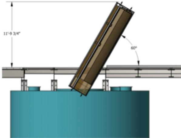
**Figure 7.4.1.** A step in the assembly sequence for the outer detector system. This shows one of the quadrant vessels at 60°, the point of maximum height above the water tank.
