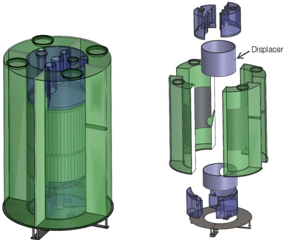
**Figure 7.3.1.** Layout of the LZ outer detector system, which consists of nine acrylic tanks. The largest are the four quarter-tanks on the sides. Two tanks cover the top, and three the bottom. The exploded view on the right shows the displacer cylinders placed between the acrylic vessels and the cryostat.
