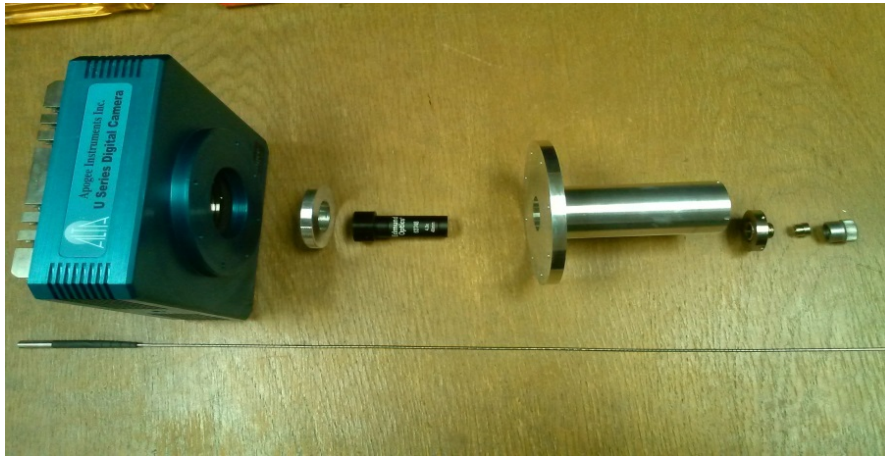
Figure 6.10.5.1. Above: Disassembled camera setup. From left, they are: camera, F-C mount converter, telecentric lens, camera/optical fiber adapter (disassembled). Beneath: Optical fiber.
