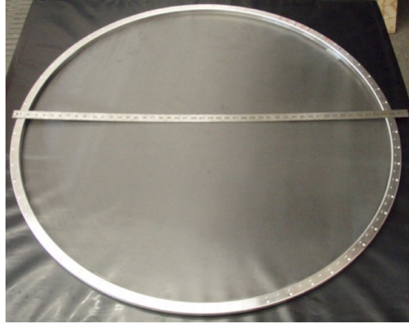
Figure 6.2.1.7. A 1.16-m-diameter stretched prototype of the LZ anode grid.
