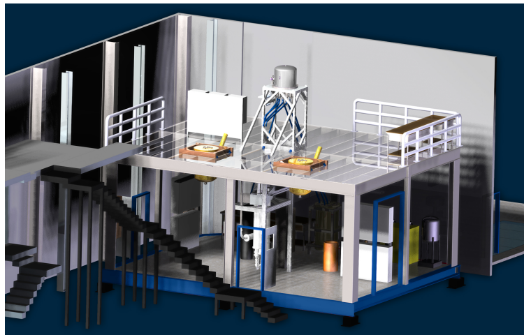
Figure 6.10.4.2. The System Test Platform housed at the former counting room for BaBar at SLAC.
